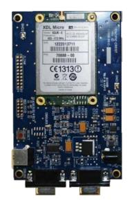
The XDL Micro test board is supplied as part of the XDL Micro Developer's Kit and is key to getting started with integration of the XDL Micro transceiver.
